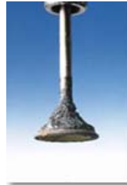
Dirty Intake Valve
